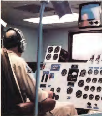
Remote control: the pilot of the aircraft in his cockpit on the ground
